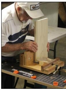
router was a 3/8" end mill. The jig was constructed so that it fit the bushing. The holding jig also held a metal pin that was considered a locater pin. The purpose was to bump the drawer panel up to the pin, push the jig and drawer panel into the router bit to make the first cut of the end mill.
