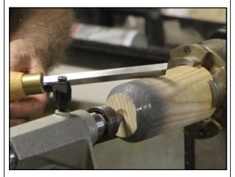
He drilled a small hole into the end of the blank that will eventually be for inserting an eyelet, once the ornament is complete.
