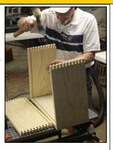
Before the drawers are glued together, one should cut off the bottom edge of one of the panels that will be to the back of the drawer. This is to allow the drawer bottom to be slid into position after the drawer parts have been glued up.
