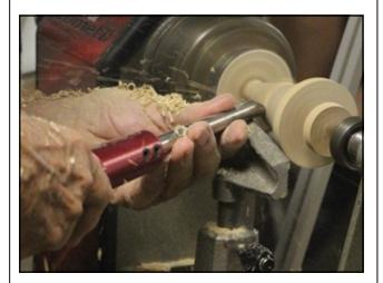
He then cut the "branches" into the side of the blank. He used a parting tool to cut each of the limb profiles.
