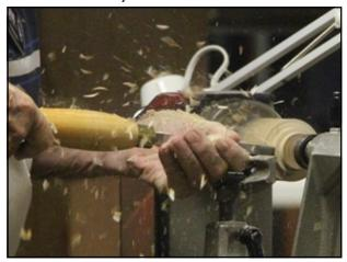
After reversing the blank he noted that the top of the tree ornament will be at the head stock of the lathe. He used the bedan to cut the bottom or base of the tree and clean up the bottom. He cut to the center or "trunk" of the tree with a 3/8" parting tool or bedan. As one is progressing to the top of the tree in the layout, the trunk should become more narrow. Hoby indicated that one should watch for catches, because that will mark up the piece.
