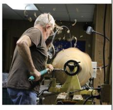
Using 1" steel Bowl roughing gouge, he establishes a rough shape.
