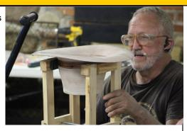
Turn the hat around, using a light you can see the consistency of the wood.
