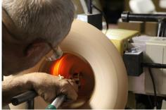
Now hollow the rest of the crown, within one finger width of the tip and the wall thickness 1/16". Use the light again, from the backside. He entered
