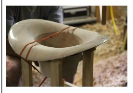
Now you can burnish the hat with a band. Then use the bending jig to allow the hat to dry in the form desired.
