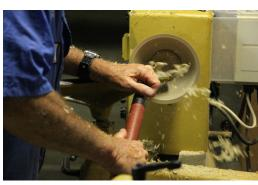
For turning the deeper bottom of the interior part of the bowl, one should use a bowl gouge with a blunt grind for that deep bottom. This will provide a smoother cut across the bottom of the piece.
