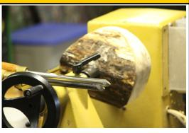
ing the bowl gouge and placing the tool edge approximately at 45 degrees to the bed of the lathe and lower the handle to make the cut. This angle of the cutting edge at 45 degrees and the lowered tool handle, will give the cutting edge the correct position to take small cuts of thin curled wood shavings and provide a very smooth surface. The cutting edge MUST be ahead
