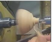
inside corner is used to gage the correct size for a tenon. The opposite outside corner is used to set the correct size for a recess. There is a small notch on the square end of the gage that indicates the depth of the chuck jaws. The gage dimensions are set so that the chuck jaws are at the most round position when grip-
