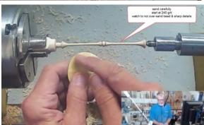
After the top half of the stem was complete, he repeated the process on the bottom half, starting at the bottom and working his way up to the bead. After he was satisfied with the stem, it was time to apply the india
