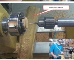
jig that fits in his chuck jaws where the contour is close to matching the curve of his base. There is also a small pin cut in the jig that centers the base in the jig. He uses the tailstock to provide support during the initial cuts to finish the base.
