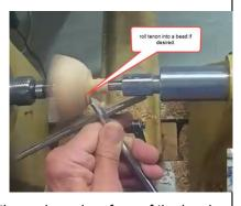
lathe and inspects the grain and surface of the bowl to determine if it would be better to leave the natural edge on the bowl or remove it. At this point, the outside surface of the bowl is done.
