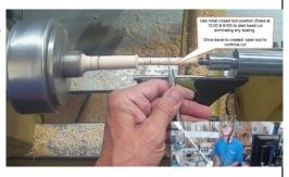
determined where the center of the stem was and the overall length. There will be a bead detail in the center of the stem. He started out with cutting a cove in the end and then turning a thin section down to the
