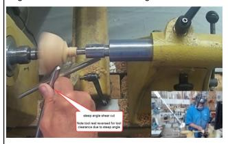
It is now time to put a smaller tenon on the bottom of the bowl to attach the bowl to the stem. Dave uses a 15/64" wrench sharpened on the top side to cut this small tenon. He sizes the tenon in an area away
