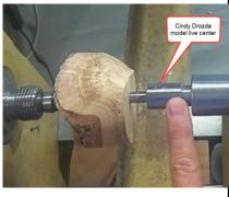
ural edge is visually balanced. When he has the blank balanced, he trues up the roundness to the new position of the blank. He then starts to shape the outside of the bowl with a 1/2" bowl gouge.
