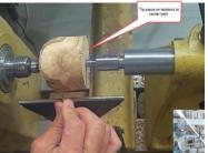
Dave was then ready to cut the tenon on the bottom of the bowl. He has made up various chuck gages that tell him what size to make tenons and recesses for each of his chuck jaws. The point of the
