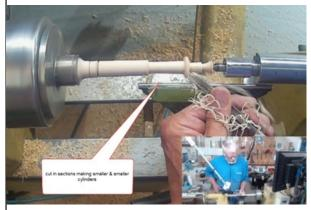
Dave then brought up the tailstock, using a cone center to support the piece. After making it round, he
