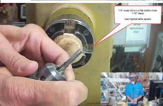
After cutting the hole, it is time to reverse the base to finish the bottom. Dave didn't use a chuck to mount this; he has made up a contoured
