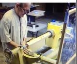
It is now time to make the two stretchers. Use the storyboard to determine the length of both the short and long stretchers. Add the length of the tenons on each end of the long stretcher and one end of the short stretcher. Before turning the long stretcher drill a ¾" hole about 1" deep in the middle of the stretcher. Make the long stretcher first using the same methods used to make the legs making sure there is a ¾" tenon with about a 45° shoulder on each end.
