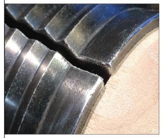
they are completely closed. When the jaws are expanded beyond a true circular form, they will still hold, but your work is more likely to turn true when the jaws make contact completely around the tenon.
