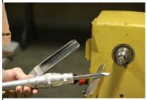
should use only the lower edge of the skew when turning along the spindle. He also suggested that one should grind off all the corners of the tool shaft. Tool steel is very hard, espe-
