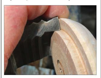
The inside of dovetail jaws, the clamping part, is smaller in diameter around the base of the tenon and larger in diameter around the end
