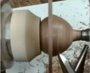
After shaping the bottom of the bowl, it is time to cut the bowl free from the wing so that it spins. Jason uses an ultra-thin micro parting tool for making these cuts. This tool has been ground special so the cutting edge is about 1/64" thick, 1/4" tall and 1/4" wide.
