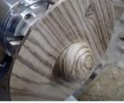
The next step is to remove the bowl from the jam chuck and then finish the top surface of the bowl. It is very important to not pull on the wing parallel to the grain. It should only be pulled off the jam chuck with
