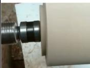
He next marked the jig at about 1/3, 2/3 from each end and a witness line across where the split will be. After this he parted the jig on the 1/3 line with a thin parting tool.
