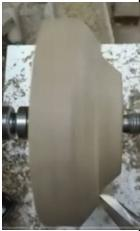
The next step was to start cutting the bottom of the wing. It is very important to make the bottom of the wing as near perfectly flat as possible. He did this by taking short stepped cuts across the bottom of the wing and then shear scraping across the bottom to blend the surface smooth and flat.
