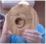
Jason started the project with a kiln dried Zebrawood blank that was about 6" diameter and 2" thick. He mounted the blank between centers and started by
