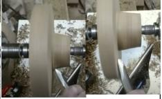
After he had the bottom of the wing to his satisfaction, he cut a tenon on the bottom of the bowl section. After the tenon was sized, he used a spindle gouge to add a dovetail detail on the tenon. Before moving on, he trued up the outer diameter of the wing.
