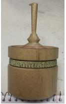
For the first box Joe first located the center of his 2"x2"x4" blank. He then mounted the blank between centers using a steb center to drive the blank. Joe
