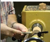
Since this was an end grain box he cut from the center of the blank to the edge of the blank to clean it up. He then used a scraper to cut a recess in the middle of the lid. He followed this up with using a skew to cut a recess on
