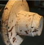
Turn the outside profile shape of the hat stopping at the top of the hatband. This can be straight or have a gentle ogee shape from the top of the hat to the hat band. The top of the hat will have a small curve inward leaving no sharp corners and leaving a tenon above the top of the hat.
