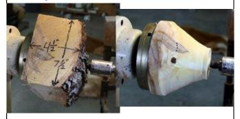
Remove the faceplate, mount the chuck on the headstock and mount the blank in the chuck using the tenon you have created. Turn the bottom of the blank flat and cut a 2 ½" mortise in the center so it can be held in the chuck. See figure below left.
