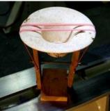
The grain must run parallel with the direction of the bend. The front of the hat and the back of the hat must be end grain sides or the hat will not bend properly and will crack.
