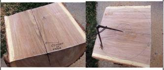
The corners of the blank can be removed on the lathe or with a chainsaw and the blank can be cone shaped prior to mounting on the lathe if preferred. See figure below.
