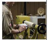
During the turning process he used a glove for hand protection and safety. He also said that if he were in his own shop, he would also be using a face shield to protect him from the chips and pieces of wood that
