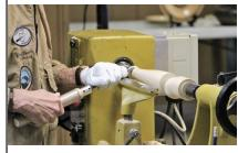
of the knob to the indent mark but leave enough wood material there to hold the bat in place. This cut should remove the offset indent hole. Use sandpaper to
