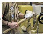
shape. Check with a calipers to make sure that you have the correct shape. Next, turn down the barrel of the bat below the ball toward the handle and knob of the bat. Do not touch the offset ball. Provide a gentle taper of the bat to the handle. Use a roughing gouge or spindle gouge to complete the handle. Use a skew to refine the surface as needed.
