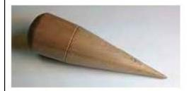
To allow for the varying diameters on a complex finial, I turned a 1  $\frac{1}{2}$ "- (38 mm-) diameter cone about 4" (10 cm) long, and it has proven to be a versatile sanding aid. I wrap the cone with a piece of sandpaper and match the diameter with the turning. Where the curve is tighter, I simply move the cone to match the new diameter. To expose fresh abrasive, rotate the cone.
