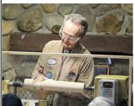
plastic was held over the center diameter of the ball, perpendicular to the bed and the lathe is running. With some hand pressure on the plastic card, he was able to melt the outline into the card.
