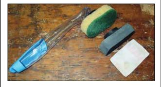
For anyone who has arthritic fingers or has trouble holding small pieces of abrasive, try a dish-mop sander. It can be used on the lathe or to sand small boards or edges. Buy an inexpensive dish mop, remove its sponge/scourer pad, and replace that with a piece of high-density foam. I glued self-adhesive hook and loop to the face. Any cloth-backed
