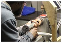
remove the drill bit from the drill chuck for safety reasons. Turn the piece around in the chuck so that excess wood can be cleaned from the other end as well as squaring up the bottom surface. Remove glue-up piece from the chuck.
