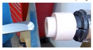
The next step was to remount the base in the chuck. He then faced off the face of the overlap with a bowl gouge and then used a rounded negative rake scraper to hollow the base to about a 1/4" wall thickness. After the base was hollowed to depth, he added a small chamfer to the overlap and finished cutting the it so that it had a jam fit with the lid.
