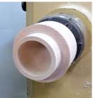
With the lid jam fit to the base, it was time to finish the top of the lid. The first step was to remove the tenon and face off the top with a bowl gouge. After the tenon
