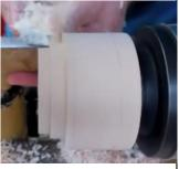
The next step was to rough and hollow the base with the bowl gouge. This was done similar to how he hollowed the lid. After roughing out, he measured the depth to make sure it was sufficient and then marked the base between the number 1 and 4 jaws of the chuck so that he could accurately remount it later.
