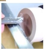
round. He then mounted the lid in the chuck making sure that it was properly lined up with the marks aligned to the number 1 and 4 chuck jaws. It was then time to fit the inside of the lid to the overlap on the base. He used the negative rake square end scraper to lightly cut the inside of the lid to almost fit onto the base and then cut a small chamfer on the opening.
