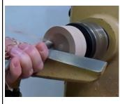
first mounted the lid in the chuck and then used a bowl gouge to face off the lid. He then hollowed out the lid with the bowl gouge. When he was almost deep enough and close to the inside diameter he wanted, he used a negative rake square end scraper to finish roughing out the lid to the sizes he wanted.
