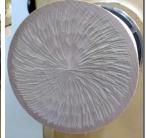
After he was done with the carver, he used a skew to cut a groove at the edge of the texture to frame it within the lid.
