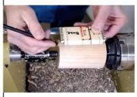
The next step was to mark the key locations on his marking gage to the blank. When this was done, he used his skew to cut the tenons on each end of the blank and cut a small
