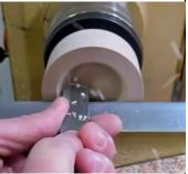
After he was satisfied with the hollowing of the lid, he measured the depth inside the lid to make sure it was close to what he wanted. It was then time to remove the lid, so he marked the piece between the number 1 and 4 jaws of the chuck so that he could accurately remount it later.
