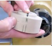
The next step is to hollow out the base. After mounting the base in the chuck, he faced off the end with the bowl gouge the same as he did with the lid. The next step was to measure the inside diameter of the lid and
