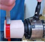
After separating the lid from the base, he used the skew to cut a small shadow line on the base where it meets the lid. This was a distinct feature that visually
