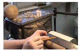
Square the ends and trim until the length and diameter are equal. The parting tool or bedan is excellent for this.
