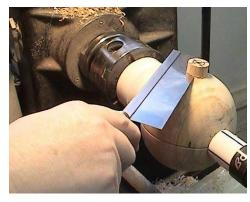
Locate the center and cut a second groove perpendicular to your first groove. This second groove must be to the exact depth as the first one without cutting any deeper. Watch the shadow along the top edge of the sphere. Turn away any material that does not appear solid down to but not beyond the first two grooves.
