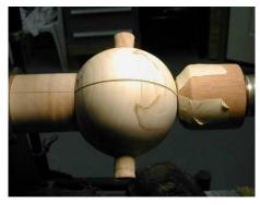
The easiest way to remove the "ears" is with a small hand saw.
