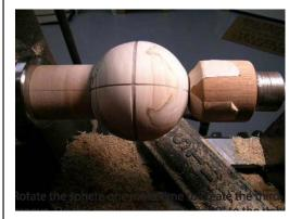
Rotate the sphere one more time to create the third grove. Do this by turning the sphere 90° to the right and keeping the first groove on the center axis. Make sure that the third groove does not extend deeper than the previous two.
