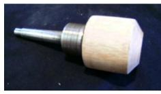
your sphere between the two cup centers. Make sure that the 1st groove is now aligned with the lathe's center axis and is parallel to the lathe bed.
