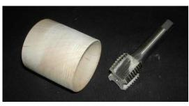
For the tailstock side, there are several options as well. If you have a live center with a removable point, you can turn a cup center with a stem that will fit into the center hole once the point is removed. If you do not have a live center with a removable point, you will need to turn a cup on a block that is drilled or hollowed to fit over your live center. The size of the cup will depend upon the size of the sphere you wish to turn.
