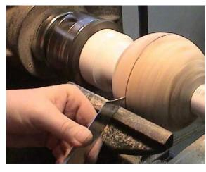
Use a detail or spindle gouge to begin rounding, starting at the corner. Be careful not to cut away the center groove or take away too much wood at the top of the curve.
