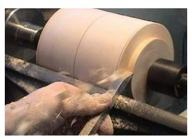
Use a parting tool to cut a slight groove on the center line.
