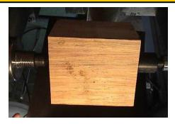
Turn the rectangular blank down to a cylinder using a roughing gouge.
