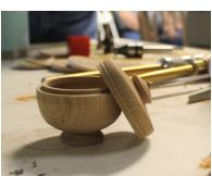
sure to cut a dovetail inside of the top lip with a recess behind it for chuck jaw clearance. This will allow reverse mounting of the base on the chuck. Reverse mount both the top & bottom pieces on the chuck to finish them.
