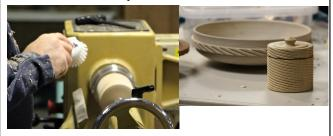
He also demonstrated Sprialing on the end-grain. Different patterns can be achieved by holding the tool at various angles.
