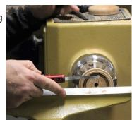
a skew or parting tool to allow reverse mounting on the chuck. It's important to leave a flat ledge at the base of the inside dove-tail so the top rest flat on the chuck jaws. When reverse mounting the top, only tighten the chuck jaws 1/4 turn after they touch the part & be very careful to note the correct way to turn the key when removing te part from the chuck.
