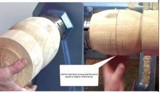
After the joint was fit, he added the bottom part to the top and used the tailstock to hold it in place paying particular attention to the fit. Pat then used a spindle gouge to smooth up the match between the two parts. It was then time to decide how to decorate and hide the joint. The first decision is to decide the extents of the detail on each side of the joint. The decorative
