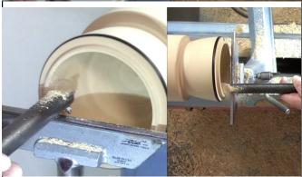
After the bottom was hollowed, Pat used a 1/2" bowl gouge to remove the bulk of the material from the outside of the bottom and to shape it with a gentle curve. After the shape was done, he used the bowl gouge to shear scrape and smooth the outside.
