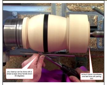
Pat moved on to shaping the outside of the top with a bowl gouge, using a bevel rubbing cut. When he was satisfied with the shape, he smoothed out the sides with a shear scrape. He next repeated the process on the top half of the bottom. After that he removed the bottom from the lathe.
