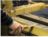
Pete then hollowed the ring from the front face using the bowl gouge & parting tool to form the rectangular walls of the hollow area.
