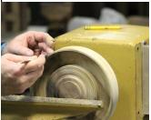
He paused to check the depth using a ruler to achieve the 1/8" wall at the bottom.
