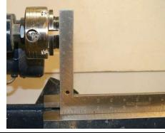
Draw a line on the lathe bed. File a shallow groove on the bed and fill the line with a permanent marker or make this mark on a piece of masking tape.
