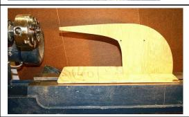
Slide the jig into the bowl until the point touches the inside bottom. The distance from the left end of the base to the line in the bed indicates the bowl bottom thickness. This bowl has a bottom about 1" thick.
