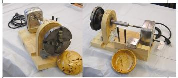
Drill into the end of the 1" (25mm) bolt so that the .375" (10mm) bolt sets .75" (19mm) into it. Drill and tap the inside of the 1" (25mm) bolt to hold the .375" (10mm) bolt with a setscrew. Loosen the setscrew when applying finish. The 1" (25mm) nut, which is also drilled and tapped, serves as a stop for the chuck.
