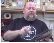
At this point it was time to set the bowl aside and wait for the paints and reactive solution to do their work. Jeff cautioned that when spraying the reactive solution, it is best to keep away from all metal surfaces (such as the lathe bed and tools) because the solution will oxidize any exposed surface that it comes in contact with.
