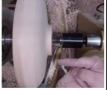
Jeff chose to use a Rubber Chucky "no nose" friction drive chuck with a Morse taper to mount the bowl. He used the indent from the live center to center the bowl on the chuck. After the bowl was mounted, he turned the lathe on at VERY LOW speed and slightly loosened the tail stock. He then held his fingers on the inside wall of the bowl and slightly shifted the bowl until it was running true and then re-tightened the tail stock
