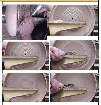
The last step is to remove the tenon so the bottom surface of the bowl is rounded off. There are several ways to mount the bowl so the tenon can be removed. They are:
