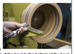
cuts from the rim of the bowl to the bottom of the bowl near the headstock. These light cuts put very little pressure on the glue joints and begin to smooth out the exterior walls.. He cautions that one needs to adjust the tool rest as needed for better control. It should be noted that the lathe must be stopped to make this adjustment. Use slow cutting techniques. Make sure to watch the areas from one glued segment
