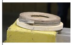
When all pieces have been assembled in a ring, he will then use a band clamp to tighten the segmented joints together. He may use a
