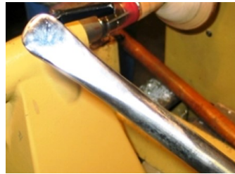
Metal tool used for metal spinning
