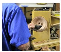
his gouge from skating across the face of the bowl. He then proceeded to hollow out the inside of the bowl using his ½" and 3/8" bowl gouges. Finally, he used a negative rake bowl scraper to fin-
