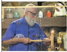
platter and wet sand it using Abranet woven sandpaper. He started by mounting a piece of cherry about 12" diameter x 1½" thick on a faceplate. He flattened the bot-
