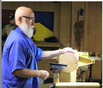
Bill started his demonstration by turning a bowl. He mounted a maple turning blank about 9" diameter x 4" thick with a worm screw in his chuck. Bill used a ½" bowl gouge to progressively remove the
