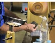
the wood so that no more of the oil soaks in. Bill then used automotive grade of wet/dry sandpaper to wet sand the outside of the bowl with mineral oil, starting with 180 grit. Bill cautioned that conventional
