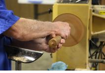
then cut a small groove in the front face at approximately the wall thickness he wanted in order to keep
