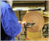
The next step was to reverse mount the platter in a chuck and cut the top surface. He started by cutting the top side of the rim and then shaped the center of the platter. After he was satisfied with the
