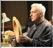
the blank must be returned back into round. There are several ways to do this, but George likes to carefully mount the rough blank using the original bottom recess and turn a new spigot on the inside of the bowl.
