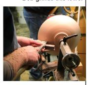
finish on the end-grain sections and less sanding. Bob prefers HSS tools over carbide for bowl turning as he feels they cut a smoother surface if used properly.
