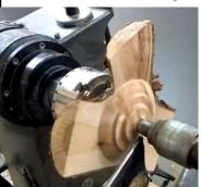
After the sanding was complete, he used a parting tool that was ground at angle to match his chuck jaws to fine tune the tenon on the bottom of the bowl to fit his chuck.
