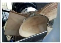
mass in the middle in order to reduce the stress in the mass. After he was satisfied with the wall thickness at the rim, he continued hollowing the bowl and removing the mass in the center, the same as
