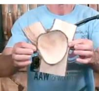
rake scraper. At this point he would remove the bowl from the lathe and use a small handsaw to remove the rest of the nub and then sand that area smooth.
