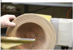
checking the depth with a gauge, small enough to insert into the chuck spaces to get to the actual middle, as to not go too far.
