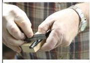
allowing the gouge to sit in the rabbet while grinding, for safety. The grind he uses is the same degree he uses for his bowl gouges, for simplicity. He ground the 3/8" bowl gouge until he had sharp
