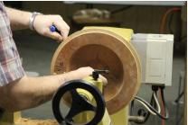
it on the chuck. He cleaned up the rim, leaving room for beading.
