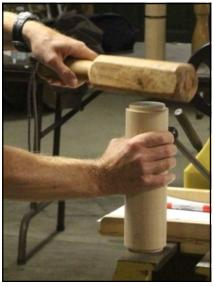
offset turning axis. He then used a protractor to mark off the radius distance of the tenon along the exterior rim of the tenon on the complete top and bottom or the blank. This produced 6 marks along the tenon rim edge. He then took every other one to acauire his three points of 120 degrees along the
