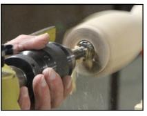
to sharpen them for every peppermill that he makes. He prefers to drill out the center of the peppermill on the lathe and uses the center point in the end of the blank to align with the tailstock ball bearing center and then tighten up the scroll chuck for the drilling process to be completed. When turning the three axis points to get the twist concept on the exterior of
