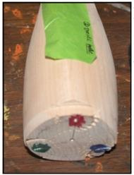
tenon edge. Dirk found that it is very easy to find the correct axis at 120 degrees by marking them with a color pen. He used red, green and blue and he also marked the other end to align the profile to be turned. He used a simple numbering system of 1,2, and 3. He would number the other end with the
