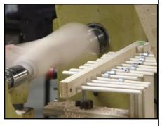
woodworking. Dirk always used a safety helmet with a shield to protect his eyes and face. He turned on the lathe at slow speed and then increased the speed until he brought up some vibration. He was able to
