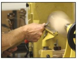
gently with the tool and took LIGHT cuts into the blank. He used a ½" spindle gouge and ground a 35 degree angle on the cutting edge. He stopped the
