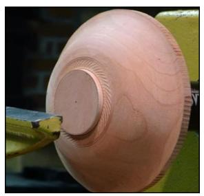
will outline the texturing with two cut lines that he made with the tip of his skew. He said that one should be careful with this texturing to make sure that the tool does not skate and cause marks where you have decided you do not want them. He uses a small brass brush to remove any chips or fuzzy remains that have been left there by the spiral texturing.
