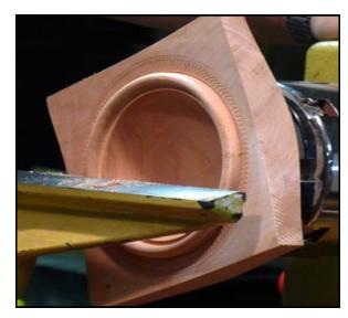
parting tool. The inside groove can be deeper. Create
