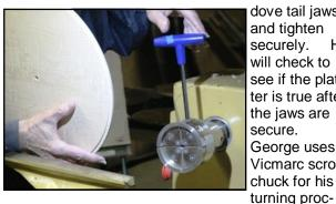
dove tail jaws and tighten securely. He will check to see if the platter is true after the jaws are secure. George uses a Vicmarc scroll chuck for his
