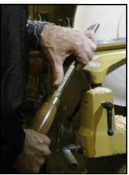
make the finishing cuts on the bottom. He will use a pull cut for this process along the side edge of the bowl gouge grind. He will use the lower edge of the grind with the groove of the gouge pointed toward the bottom of the platter. The tool handle will be held low and pointed at the persons' thigh. This angle of the tool will give the cutting edge about a 45 de-
