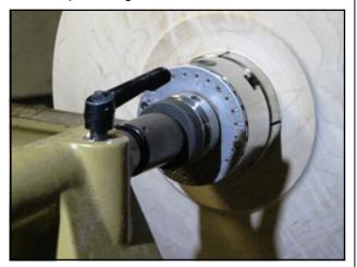
assured a centered fit on the rubber boot on the tailstock. At this point, he turned on the vacuum to mount the platter. He then removed the scroll chuck and the tailstock adapter. He turned the speed way down on the lathe so that the piece was moving slowly. He said that one can make a series of coves and beads or cut signature lines into the bottom with a 3 point tool that is made from 1/4" or 3/8" round steel stock. George uses a number sys-
