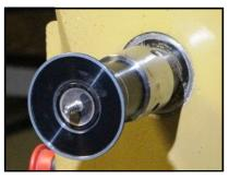
flat of the screw chuck. If the turning blank for the platter is to thin, then he will use some wood washers in between the blank and the chuck to take up some of the screw thread space. He does not want the threads of the screw to protrude into where the bottom of the platter will be. Normally the screw threads are about 3/8 inches in diameter, so the hole that is drilled in the blank needs to be of a smaller diameter, like 5/16" or less.
