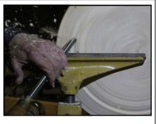
shaped and he will use parting tool for a very accurate and delicate cut. This cut also has the purpose to remove some of the warp of the rough blank from the top side. He also said that when making platters, one always is working with curves. He has found that by using a short length of chain and hold-
