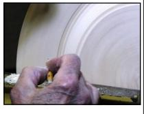
that is severely tapered, then the bowl area will be shallow. George likes a slightly rolled rim with the thicker part near the edge of the rim. He likes a 1/32" taper from the high part to the rim.
