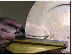
platter, one should roll the tip to get a better cut. Remember that the rotating center is moving very slowly, compared to the outside rim speed of the piece. Take lighter slower cuts as one approaches the center of the piece to get smooth finish cuts. When the thickness has been reached, then make final thin cuts to bring it to the desired finish and blend everything together. Remove the platter from the chuck.
