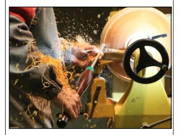
Finally, he made the finishing cut on the inside of the bowl. He tapered the wall thickness from about 3/4" at the top to about 3/8" at the bottom of the side wall of the bowl.
