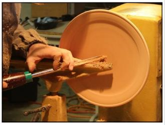
He then cut the inside wall of the plate to a gentle curve to blend in with the bottom. When he was satisfied with the inside shape of the plate he made a few finishing cuts to get the best surface possible prior to sanding.
