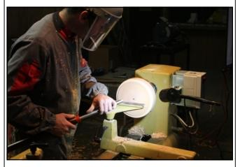
While doing this he made the sidewall thickness of the bowl about 1/2". As he moved into the depth of the bowl he cleaned up the inside surface of the bowl. He repeated this process until he had the bowl down to the desired depth with a bottom thickness of about 1/2". He made sure that when he was coring the bowl and finishing the side wall that he made light cuts to reduce the risk of snapping off the tenon. After he had the inside cored out he finished the bead detail on the rim of the bowl.
