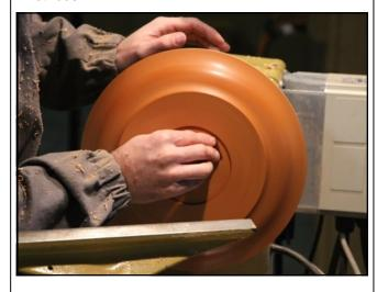
After the bottom of the plate is complete to his satisfaction, Glenn removed the faceplate from the piece and mounted it in the Vicmarc chuck. He then trued up the face of the piece about 2" in from the outer edge. He then removed the wood from the center of the piece and made the bottom wall thickness about ½".
