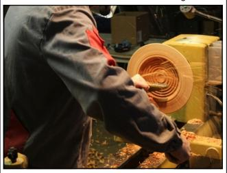
and finishing the side wall that he made light cuts to reduce the risk of snapping off the tenon.
