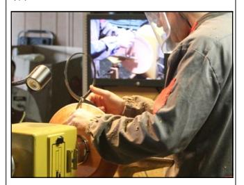
He made sure to make the bottom of the plate slightly concave.
