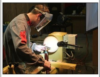
He then cut in a bead detail on the outside corner of the top rim of the bowl. At this point he added a tenon to the bottom of the bowl to fit the Vicmarc chuck.
