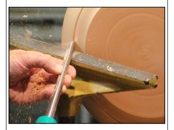
After the ogee is complete he cuts a recess in the bottom so he can mount the plate in his chuck. Glenn uses Vicmarc chucks with dovetail jaws for mounting is bowls and platters. He uses a square edge scraper for cutting the recess and then a skew chisel with a 77° angle cut on the end for cutting the dovetail. The
