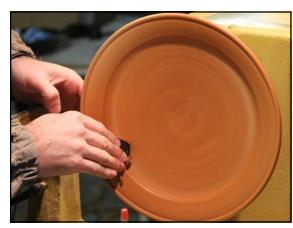
Again, he sometimes leaves the plate mounted in the chuck overnight and then dry sands the inside of the bowl in reverse up to 800 grit. He then applies a final finish made up of 80% mineral oil and 20% beeswax. The number of coats of the final finish is decided on as he progresses with the finishing.
