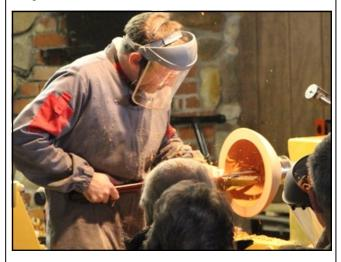
When the inside shape of the bowl was done he moved to the outside. He made a push cut to make the bowl round as it also may have gone oval during the kiln drying process. As he was completing the outside of the bowl, he used a push cut that was done with a  $\frac{1}{2}$ " bowl gouge at a shear cut of about 45° and produced a very fine shaving.
