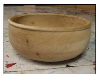
At this point he would sand the bowl through the grits up to 320 grit. Glenn did not finish sand the bowl during the demonstration. He then discussed various methods of reverse chucking the bowl (vacuum chucking and jam chucking). For the demonstration he set the bowl on a cushion on the jaws of the chuck and supported it with the tailstock. He then removed as much of the tenon as he could. After the tenon was
