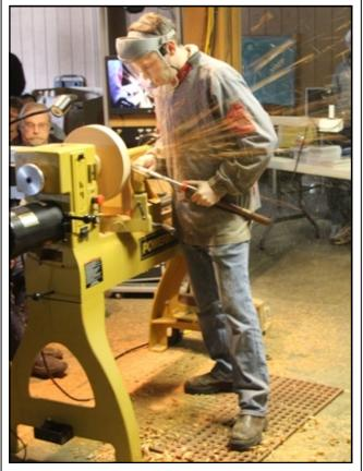
After the sides were turned, he turned a tenon on the bottom of the bowl that would fit in a Vicmarc chuck. Glenn prefers putting a tenon on the bottom of large bowls because it is stronger than a recess and will be a better mount when coring out the bowl. He is not concerned with the finish on the bottom and the tenon because that will be eventually removed. He used a
