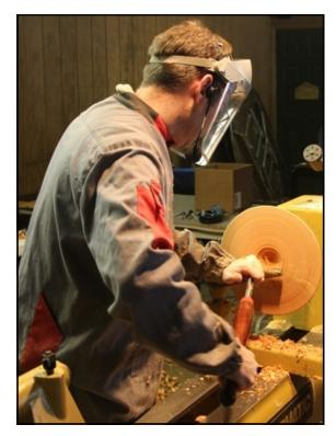
While doing this he made the sidewall thickness of the bowl about 3/4". As he moved into the depth of the bowl he cleaned up the inside surface of the bowl. He repeated this process until he had the bowl down to the desired depth with a bottom thickness of about 5/8". He made sure that when he was coring the bowl
