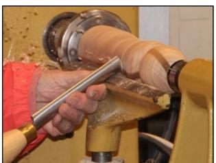
Hoby indicated that one should watch the horizon on the top of the spindle body when doing the turning as opposed to the location of where the tool cutting edge of the gouge meets the wood. He also turned a small radius on the bottom edge to provide a rounded edge where the pepper mill meets the table surface. Hoby sanded the piece with 120 grit and then requested some 80 grip paper to sand it
