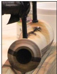
As mentioned above, oak is a very poor wood to try this burn pattern because the electrolyte will drop into the grain grooves of the oak and will stunt the burn pattern. Sometimes he will use bleach to lighten the wood and thereby getting more contrast
