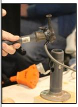
Hoby made two post electrodes that will touch at either end of the artistic burn pattern areas. These consisted of two pipes that stood vertical on a metal base and there is an attached arm that extends horizontal from the vertical pipes to touch the turned item. Hoby recommended that a foot pedal on/off switch should be used to start and stop the process.
