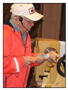
He placed the ball in the chuck and then rounded over the ball with a 3/8" spindle gouge. He made sure that the area next to
