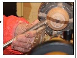
the tenon was at a 90 degree angle. He then made a counter bore in the nut or tenon to house the grinder mechanism and rod.
