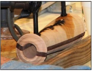
The electrified burning process is slow but continuous as it burns its way through the wood. The electrolyte provides the path for the electrical burn pattern.
