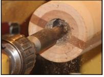
grinding mechanism. He used a 1 1/16" Forstner bit and placed it in the drill chuck that was mounted in the tailstock.
