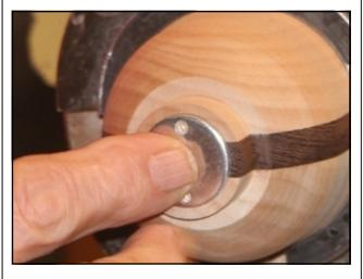
He drilled a ¼" hole in the center of the ball and then removed it.
