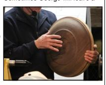
due to the drying or warping out of position or if he wishes to make any refinements to the bottom. Then he can remount it in the bottom recess and turn the interior thickness away to have a very clean and true interior.
