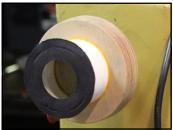
both ends of the pipe on the lathe. Then cut a groove ¼" to 3/8 inches deep into the double thick plywood and then to match the wall thickness of the pipe. This section of pipe can be glued into
