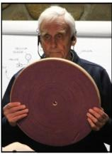
together, and the ends trued up, turn a flat true surface on the inboard side. Glue a large sheet of closed cell foam onto the surface of the chuck. This chuck would be ideal for platters and flatter turnings. But one needs to be careful to use the bleeder valve to release some of the vacuum on these large turnings.
