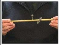
You could use a lamp rod system to carry the vacuum through the headstock. You would use rubber washers to seat the rod at each end of the spindle. You would also have to use a ball bearing and a ½" npt
