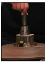
mounted into the indent in the bottom of the bowl. That should center the bowl in position to finish turn
