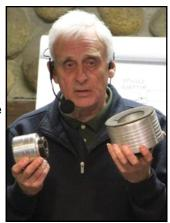
This vacuum system and chucks takes the place of the Cole Jaws that can be
