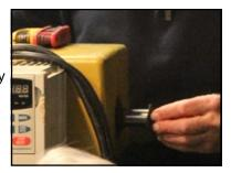
stock and it has a bearing that rotate with the headstock revolutions. It should be noted that this adaptor will need to fit the threads or shaft that is on the outboard side of the lathe. Again, George warned
