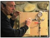
that one must be able to regulate the amount of vacuum or you will crack the thin walled vessels. The vacuum pump gauge will give you some indication of the amount of vacuum that you are pulling, but you
