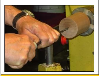
You now hollow out the interior so that it is close to the finished opening that you desire. The reason Howard does this, is so that as you are cutting the tenon for the lid, the piece may shrink slightly and then the lid will not fit at a later time.
