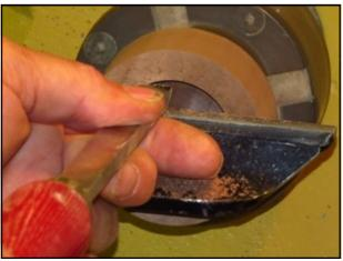
He stated that one can make an alignment of the level tool at the point of the tailstock. This would give a very true and accurate cut on the interior part of the lid. He then sanded the lid from 120 grit, down to 220 grit, so that there would be a nice surface.
