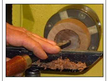
He used the upper left edge of the scraper to cut the walls to size.
