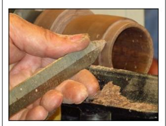
He now cleaned up the exterior walls of the box bottom to the proper thickness. He then sanded the interior of the box sides and bottom to a desired finish. He then applied wax to the interior and then buffed the walls and bottom to his satisfaction. Now he parted the bottom off of the waste block. He made a tenon on the waste block so the bottom could be reversed in the jamb chuck. He aligned the ball bearing tailstock to provide accuracy in turning the bottom.
