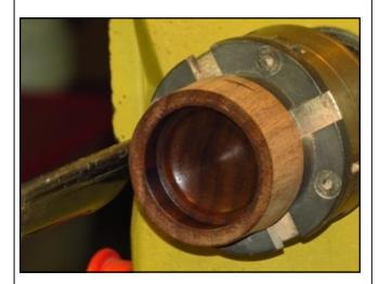
Howard now turned to finish the exterior of the box lid. He used a depth gauge to check the depth of the interior of the lid and them marked that depth on the outside of the lid. He cleaned up the exterior of the lid sides and began to shape the top of the lid.
