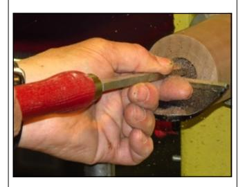
Howard uses a negative rake scraper to clean up the walls and interior of the box. He uses a depth gauge to measure the depth of the interior and makes an obvious mark on the exterior of the bottom blank.
