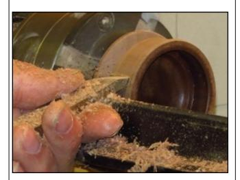
He made a tenon on the waste block so that the lid would have a friction fit to hold it in place while he fin-
