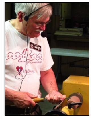
chuck and centered it up with his tailstock and ball bearing center in the previously made indent.
