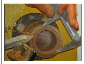
He cautioned that one should remove small amounts of wood with the tool until the lid fits. He made mention of the fact that when one is removing wood from one side you are actually removing twice as much wood over the whole piece or fitted lid tenon. He stopped the lathe and check the fit often until he had it correct.
