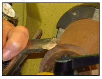
He parted the lid or top of the box off with a parting tool. He said that normally he uses a saw to remove that part of the blank.
