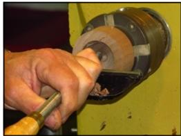
He said that you could leave a small nipple in the roof of the lid as a decoration center. It is tough to remove that nipple and thought that it would be a nice added feature. He used a scraper to clean up the walls and top of the lid.
