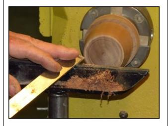
Sand all parts including the bottom and apply the wax finish as before. Any remaining nib or nipple on the bottom can be removed with a sharp knife and then sand the area to the desired finish.
