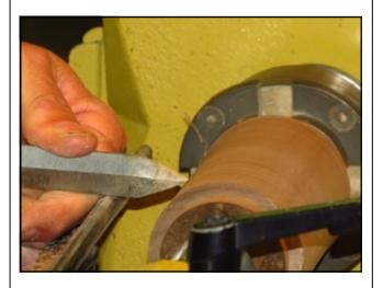
Howard removed the remaining blank and placed the lid blank into the chuck. He stated that the walls of the lid had to be parallel to each other. He used a spindle gouge to remove some of the wood and get to the full opening of the lid.
