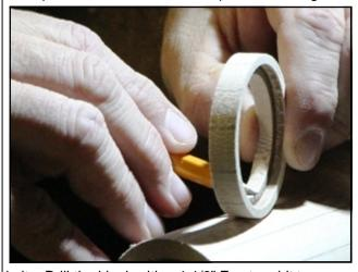
in it. Drill the blank with a 1 1/8" Forstner bit to a depth of about 3 ½ inches. Clean out the drill hole of wood chips so that the drill will not bind in the hole. Place a ball bearing center in the tailstock and then turn down the exterior diameter to 1 ½". The rings should slip over the backbone and fit loosely.
