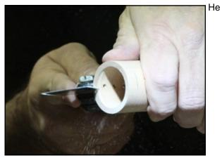
used 1/8" wood dowel rods as pins and glued them into the drilled holes. He said that they had to be long enough to get to the outer edge of the back-
