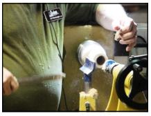
above, [make rabbet cut and then part away], until all six rings have been cut from the blank. Clean up the rings with sandpaper so that they are free from wood chips or slivers. He used a Dremel tool to cut a 3/16" groove in each ring.
