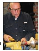
step would be to spin the metal with the tool, all the way from the center to the outside edge and then back again. The metal will "flow" or stretch along
