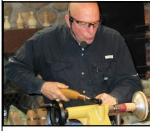
In metal spinning, the speed of the 6 inch disc should be about the same as in wood-turning. Try the lower speeds at around 1200 rpm. If you move to higher speeds then there will be increased friction and this will work harden the piece faster.
