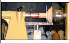
Make sure that the threaded screw center is held securely in the jaws of the scroll chuck. Then hand spin the blank onto the threads of the
