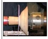
scroll chuck and the tailstock with the 'follow block' in place. Use slight pressure to hold the disc in position. Turn on the lathe to spin the metal disc. Use a wood stick to push on the edge of the metal disc to align it to spin true. Then use a lubricant to
