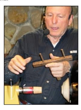
For the metal discs, Dave indicated that you need non ferrous metals, such as aluminum, copper, pewter, or brass. Metal discs can be purchased in different thicknesses. The thickness needed for metal spinning is as follows.....Aluminum, 18-22 gauge..... Copper, 20 -26 gauge.....Brass, 20-26 gauge.....and Pewter, 14-20 gauge.
