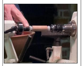
t should be noted that he used some tapered polyester bushings to hold the pen barrel in place. These were used because the CA glue will not stick to the surfaces of the polyester bushings. If wood or metal bushings are used, then you may very easily glue the bushing to the pen barrel and have a very difficult time separating the two from the barrel. It should be noted that Acetal or Delron are trade names for these polyester bushings.
