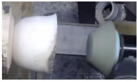
It is now time to shape the stem from the bowl to the base. This should be done in short increments so as to maintain the strength in the stem. As the stem is
