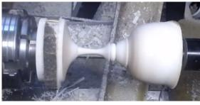
approximate top of the base. When the top of the base is defined, finish the stem and the top of the base and blend the two together. If the base is going to have a finished edge, now would be the time to do the finish-
