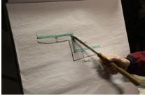
that depending on where the chuck was made, it may turn to the right to open or turn to the left to open with the use of the chuck wrench. He recommended using the letter O with an arrow showing the direction of opening and a C with an arrow for the direction of closing the jaws. He said that this might prevent a piece from falling out of the chuck and
