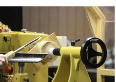
to about half the thickness of the blank. Bring the base diameter to the bottom of the bowl design. Use and up sweep shape for the wings. This is a
