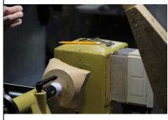
pull cuts toward the bottom of the feet on the corners. Cut a tenon on the bottom of the bowl. The tenon will later be removed and the piece will stand on the four feet on
