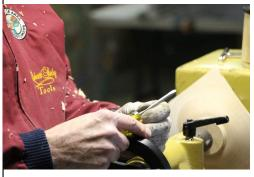
to the remaining nub. Jamie had made a small scraper out of an old screwdriver. The blade was ground away and a round scraper tip
