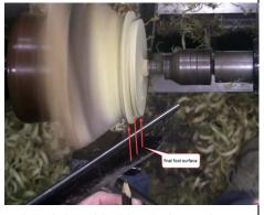
ons were removed and the side blended together to finish the shape of the side of the bowl. The next detail was to add the foot of the bowl. David cut a slight undercut around the foot to raise the bowl when it sits on a table. He followed this up with a final cut on the side using a shear scrape. Finally, David used a 3/8" detail gouge to carefully remove the nub on the bottom.
