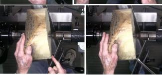
The next step was to start the turning. After making sure that the rotation of the blank did not interfere with the toolrest, he started by making the bottom flat. David used a bowl gouge to do almost all of the work. When he was roughing out the shape of the bowl, he rolled the flute over about 45° and cut with
