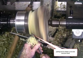
After the shear scrape on the side, he used a parting tool and 3/8" detail spindle gouge to shape the side of the bowl down as close to the chuck as he could.
