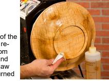
Once the exterior of the platter is finished, remove the blank from the screw chuck and mount it in a four-jaw chuck using the turned dovetail recess.
