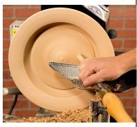
depth often to prevent making the sidewall too thin or worse, turning through the side. Leave about 1/4" of thickness between the bottom and dovetail recess.
