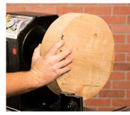
platter onto the chuck. The blank should seat firmly against the chuck. For increased safety, use the tailstock and revolving center to support the platter while rough turning and shaping.
