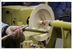
material from the heel of his gouge at the grinder to prevent "bruising" the wood fibers as he transitions the cut at the bottom of the inside.
