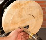
Next, turn a 1/4" deep dovetail recess to fit your chuck jaws when used in the expansion mode. Hint: Use a skew chisel flat on the tool rest, like a scraper, with the long point cutting and forming the dovetail recess. Turn a foot ring around the recess ar-
