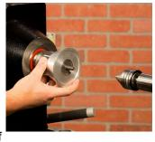
the blank is less than 2" thick, drill the hole 3/4" deep and make a 1/8" thick spacer (the same diameter as the screw chuck) to shim the blank. Now, mount the screw center chuck onto the lathe and screw the
