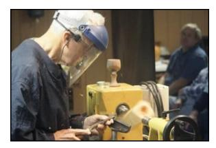
He then mounted the work piece between centers on the offset flat surfaces that he cut on the band saw. Care was taken to spin the work piece to confirm proper clearance to the tool rest.
