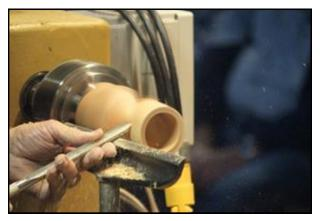
George then remounted the piece in his scroll chuck, making sure that he was oriented to the marks he made on the piece earlier. He explained that he sometimes uses a cone center in the tailstock to support the piece. He then used a spindle roughing gouge to carefully remove the material over the length of the piece, taking special care in the middle where the center offset groove is. He turned the entire piece so that it was round.
