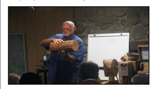
then there is a possibility that it will be out of round and cause serious vibration to the lathe. The bowl blank may be mounted off center, or there may be more dense wood at one end of the blank. Always stand to one side, away from the bowl blank, when turning on the lathe.
