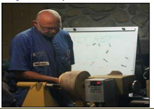
will determine how the bowl will finish out. If you are turning an end grain bowl, then the sides will be weak but the bowl will not distort when it is drying. If you turn a side grain bowl, or the grain running perpendicular to the lathe bed, then you will get some distortion but the sides of the bowl will be very strong.
