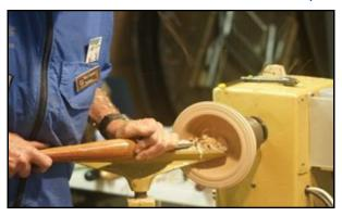
proximately 1/3 of the top rim surface. When creating the bottom, one should put a straight tenon on the piece but that it should be at exactly 90 degrees where it transitions to the curvature of the bottom of the bowl. This is so that it will fit exactly into the jaws of the scroll chuck. Any other angle in that corner will not allow the jaws to hold the work correctly.
