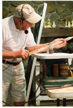
To clean up the tapered spiral spindle, he uses an oscillating spindle sander. He uses a thin sanding spindle to get into the grooves that he cut in the tapered design. He hand holds the cane against the sander and he works the grooves to remove any
