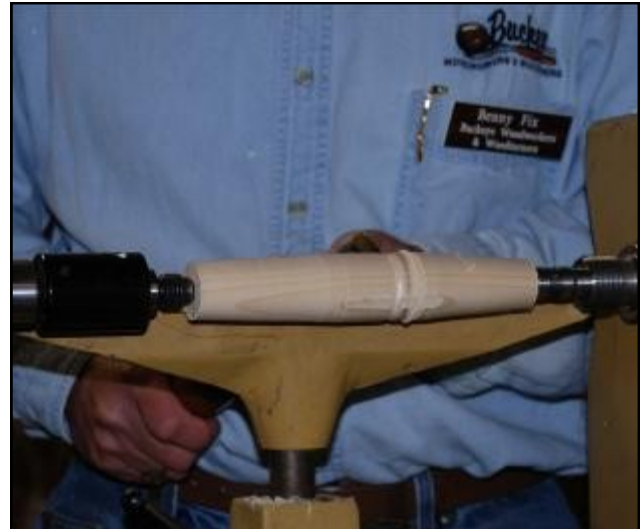
Ben demonstrates a straight cut with a skew
