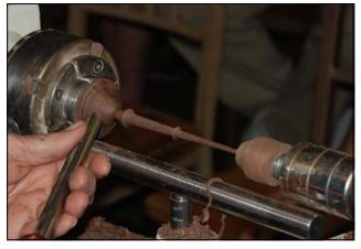
Hoby uses a sharp 1/4" spindle gouge to turn the desired shapes. Hoby's thin finial was between 6" to 8" in length. When the thin finial is turned to completion, one can sand and add some finish of choice. At all times one should be careful not to use aggressive pressure for fear that the finial might break. When the finial has been shaped and finished, he reversed it into the scroll chuck hole and into the Morse Taper #2 opening.
