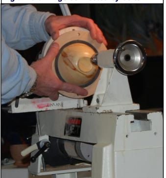
Another adaptation of this method is to use a plastic pipe coupling and cover it with fake chamois. Glue the PVC pipe mounting over a turned wood blank with a recess. This could be used in a scroll chuck or with a captured nut in the wood backing, it could be screwed onto the threaded headstock.
