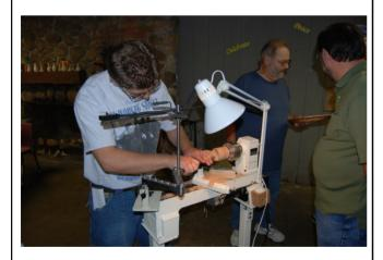
Larry McCardel used an articulated arm to show hollow turning on a mini lathe. This arm has a large range of mobility at the lathe to do interior hollowing of vessels. He used HSS tips of 1/4 inch and 3/16 inch size for his hollowing techniques. He stated that he aligned the tip to be at the center line of the wood blank. His articulated arm was called
