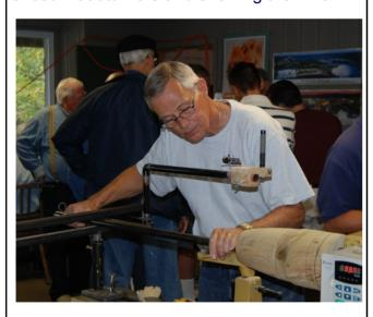
to cut beads on spindles. He used the heel of the skew and demonstrated the movement of the tool on the wood to roll the beads with very little sanding needed to complete the quality of the piece. He also demonstrated the use of the smooth plane cut whereby he held the tool in a rather flat position and cut across the wood blank to acquire a smooth
