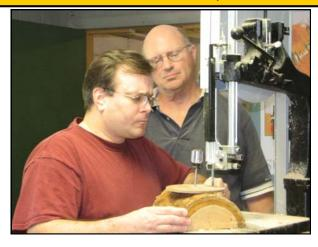
Here Jerry Schaible watches as Bob Hasenyager uses the band saw to cut a round turning blank from half a log using a round plywood template as a guide.
