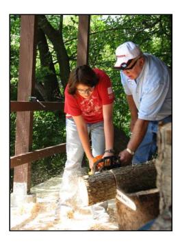
Above, Larry McCardel provides instruction to Olga Eliseeva on proper chain saw usage cutting off a length of log. The next step will be to cut that piece in half length wise through the center of the log.
