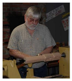
For the stand off piece, Joe would cut a tenon on the front to be inserted into the turned sconce. He would cut two dowel holes in the other end for insertion into the back board.
