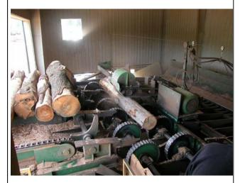
The logs enter the mill here at the de-barker where the bark is all stripped away and the log is scanned by a sophisticated metal detector.
