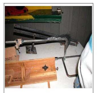
The use of hollowing tools with laser lights to determine the wall thickness. (Both a large and a small version were displayed.)
